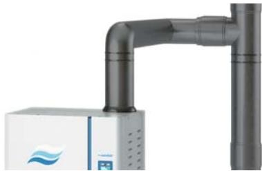
The lower flue gas temperature, created by the condensing technology, allows the use of plastic rather than stainless steel flues. This reduces the installation cost when compared to non-condensing gas-fired humidifiers.
