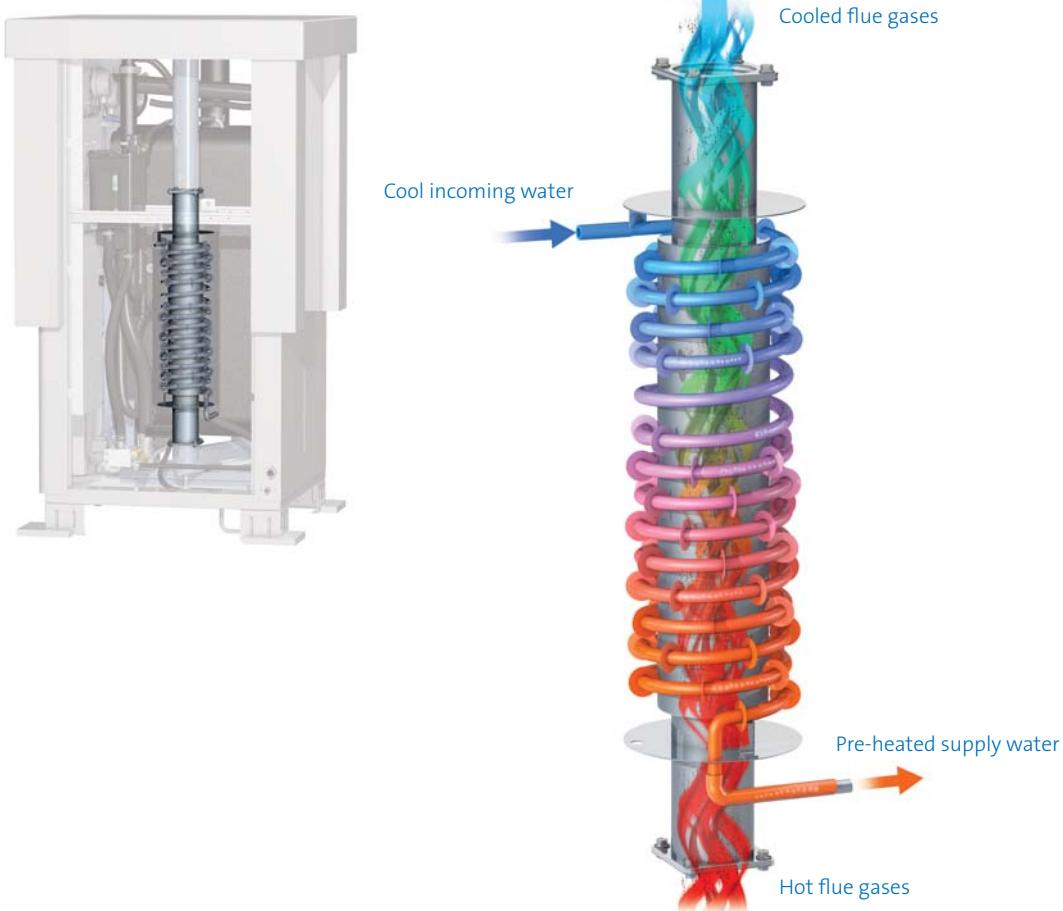
Heat is recovered from hot flue gases into the incoming supply water to save energy
